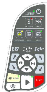
For convenient positioning close to the patient (e.g. for adjusting the detector height for chest exposure)
